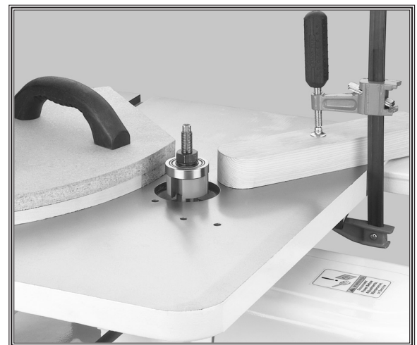
Figure 36. A piece of wood clamped to the table can serve as a starting block. (Guard not shown for clarity).
